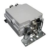
Dual Band Tower Mounted Amplifier, 2100//2600, 12 dB, 2 BTS & 2 ANT ports, AISG with 1 RET conector (1 device with 4 sub-units)
