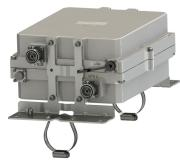
Dual Band Tower Mounted Amplifier, 800//900 MHz, 12 dB, 2 BTS & 2 ANT ports, AISG with 1 RET connector (1 device with 2 sub-units)
