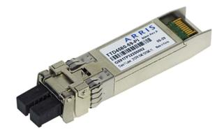
The TTD4540/TTD4580 family of modules features a very low jitter contribution, resulting in extremely clean, high-quality eye patterns. The module's metal enclosure ensures rugged durability and improves FCC EMI test margins. This emission and ESD control are particularly important in applications with sensitive multiport hubs and switches. The modules, which dissipate less than 2.8 W, are supplied with a duplex LC connector.
