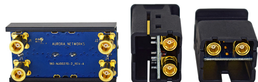
Plug-in modules bottom view, showing SMB connectors
