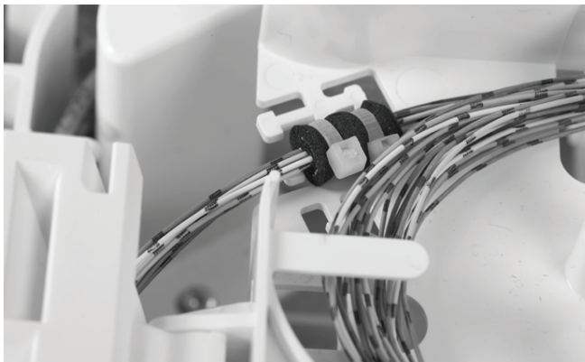
5.6 Install the foam at the position on the patch tray and secure with 2 tie-wraps as shown on the picture.
