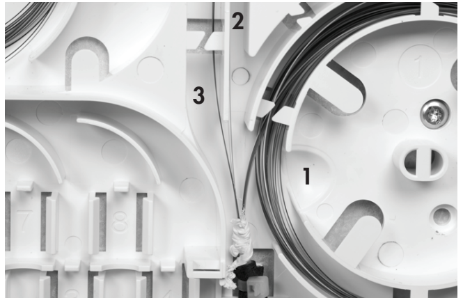
2.6 Store the unused looped fibers in the storage area.
