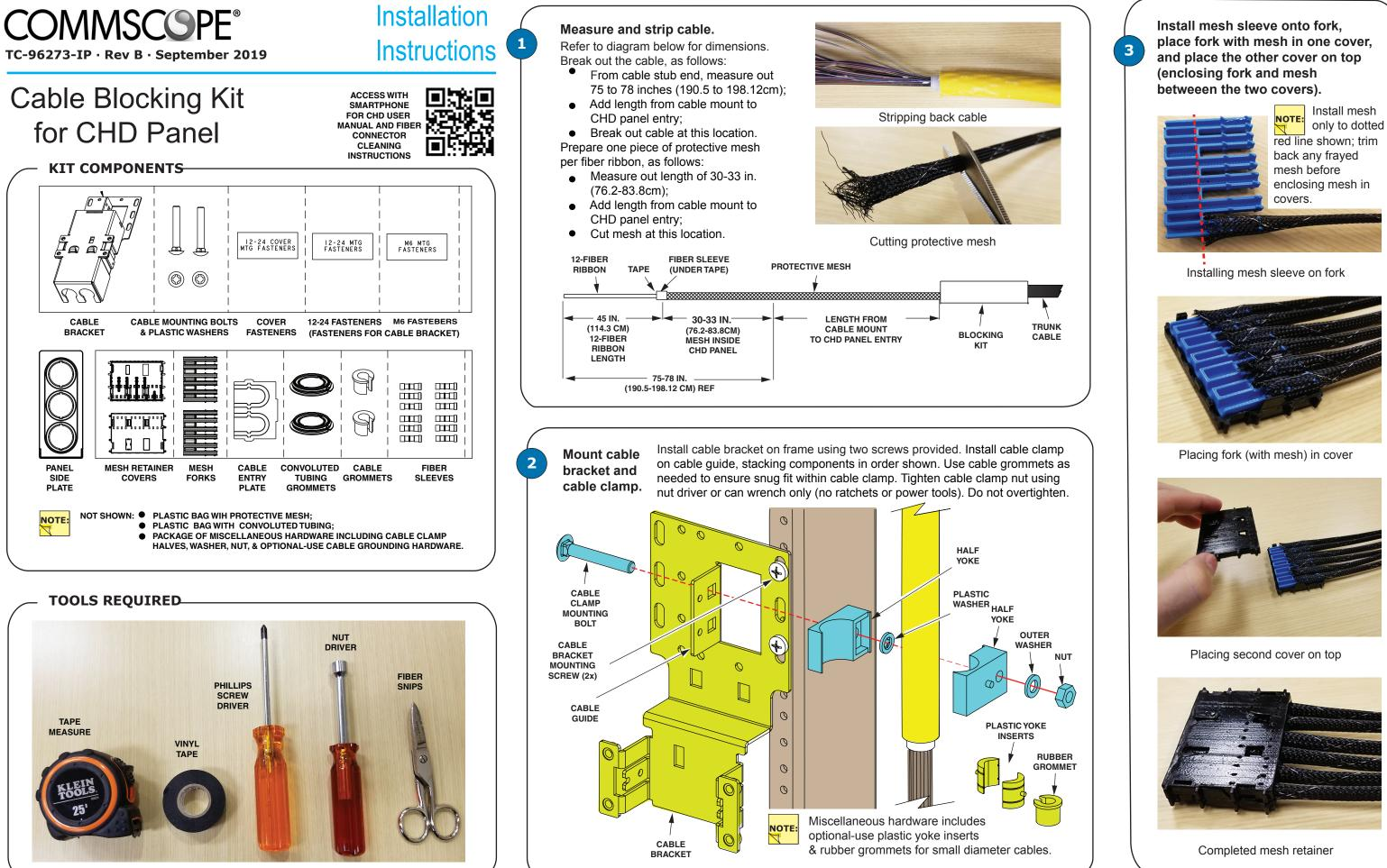
Snap the mesh retainer into the bracket, draping ribbons to outside.
