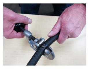
3. Remove the cut section of armor from the cable.
