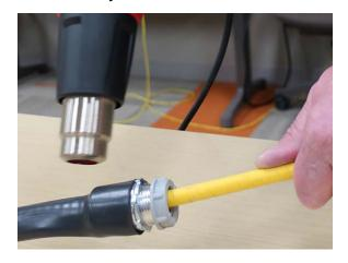
Note: The heat shrink is adhesive lined so it is normal to see a small amount of adhesive leaking out at the edges of the tubing.
