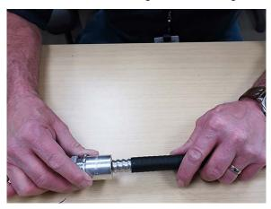
Slide the heat shrink tubing over the rear of the armor fitting until it reaches the flange at the end of the armor.
