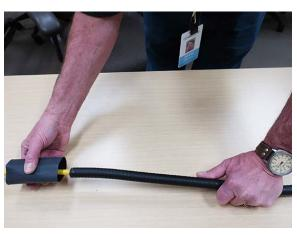
6. Slide the heat shrink tubing up past the cable armor and out of the way.
