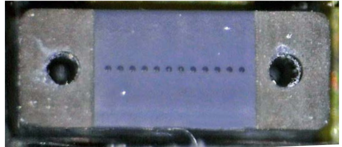
Example of HMFOC Endface with Dirty Pinholes
