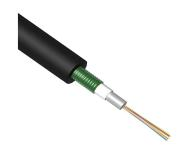
Fiber OSP cable, 6-fiber, OS2, HDPE, loose tube, 6 fiber, gel-filled, Singlemode G.652.D and G.657.A1, 1000 m, Meters jacket marking, Black jacket color
