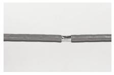
1 Remove outer PE jacket over a distance of 40 mm.
