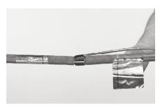
10 Apply the aluminium foil to the cables, positioning the blue line at the mark of the bond length. Smooth the aluminium foil with a blunt tool.
