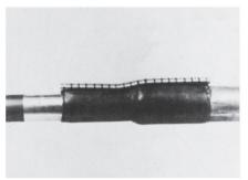
**15** Pressurization can be carried out when the sleeve has reached ambient temperature.
