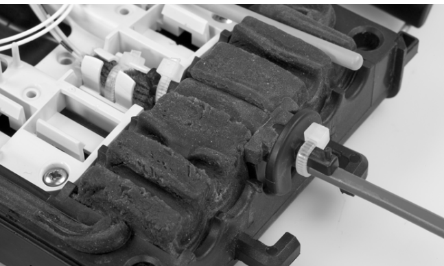
3.2.4 Click the KTU into the organizer and install the gel insert(s). Fix the insert(s) on the cable with 2 tie-wraps.
