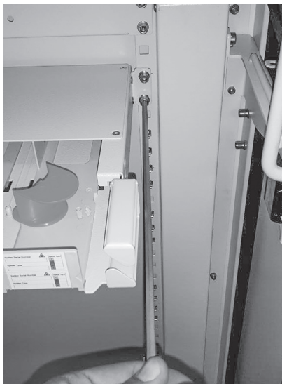
5.3 Hold shelf in place and install onto the other side of the cabinet.
