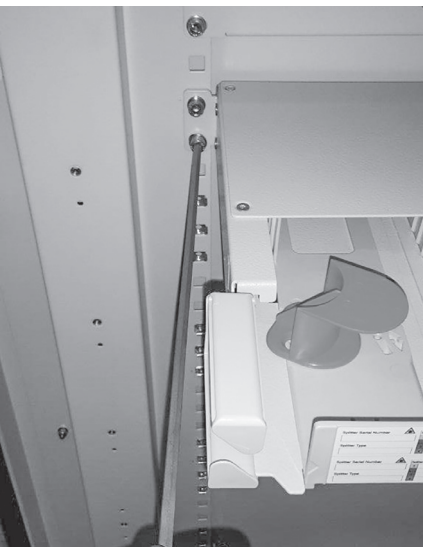
5.4 Fixate with the remaining screws.
