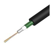
Fiber indoor/outdoor drop cable, LSZH, Gel-filled Central Tube, CST, 24 fiber, Multimode OM3, Meters jacket marking, Black jacket color
