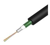
Fiber indoor/outdoor drop cable, LSZH, Gel-filled Central Tube, CST, 6 fiber, Multimode OM4, Meters jacket marking, Black jacket color
