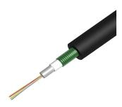
Fiber indoor/outdoor drop cable, LSZH, Gel-filled Central Tube, CST, 12 fiber, Multimode OM3, Meters jacket marking, Black jacket color
