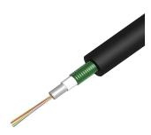
Fiber indoor/outdoor drop cable, LSZH, Gel-filled Central Tube, CST, 6 fiber, Multimode OM3, Meters jacket marking, Black jacket color
