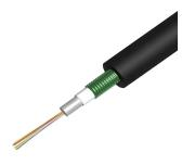
Fiber indoor/outdoor drop cable, LSZH, Gel -filledCentral Tube, CST, 6 fiber, Singlemode G.652.D and G.657.A1, Meters jacket marking, Black jacket color
