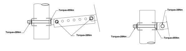
Detail 'A' Figure 6. Setting mechanical uptilt
