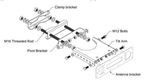
Figure 4. With Tilt Arm Mounting Bracket Exploded Assembly
