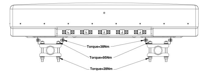
Figure 2. Fixed Downtilt Mounting Bracket Assembled to Antenna & pole
