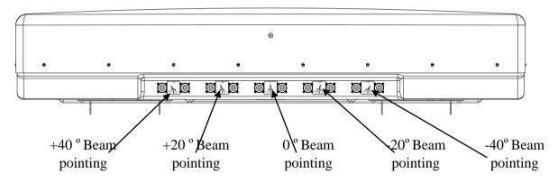
Figure 7. Arrangement of connectors on the base of the antenna.
