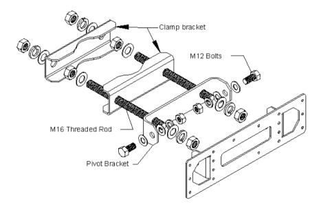
Figure 3. Fixed Downtilt Mounting Bracket Exploded Assembly
