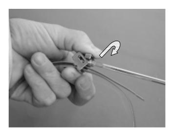
Step 4 Tighten the screw along the band up to the required strength (max 5 Nm) by means of a screwdriver.
