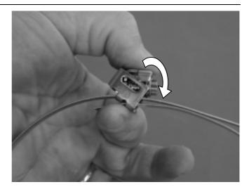
Step 3 Rotate the screw toward the band while pressing.
