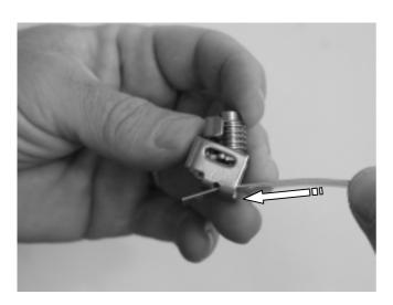
Step 1 Insert one terminal of the band into the lower slot of the buckle.
