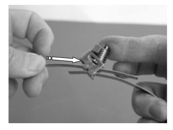
Step 2 Insert the other terminal of the band into the upper slot of the buckle
