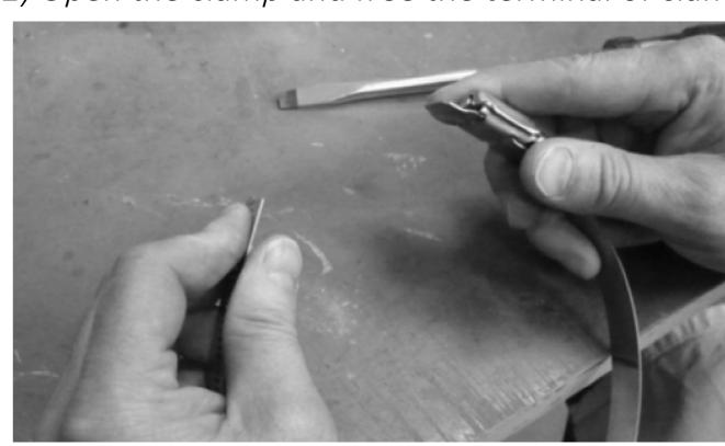
4) Insert the free terminal of the clamp into lock and tighten the screw (along the band up to the required torque MAX 5NM while mounted on the pole) by means of a screwdriver.
