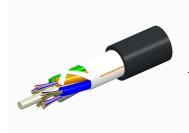
Fiber OSP cable, TeraSPEED® Single Jacket All-Dielectric, 156 fiber, Gel-Free, Stranded Loose Tube, Singlemode G.652.D and G.657.A1, Feet jacket marking, Black jacket color
