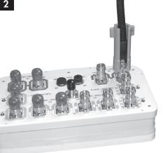
Slide the tool downwards over the coupling nut until the nut is completely covered and engaged by the tool.
