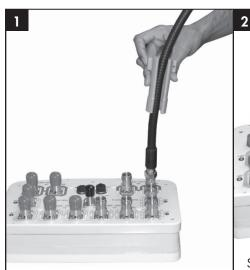
Push cable through the tool slot with hex nut wrench portion of tool facing device.
