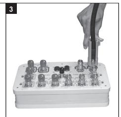
Rotate tool clockwise until it starts skipping over the coupling nut. The TW-4310 wrench can be used for additional leverage.
