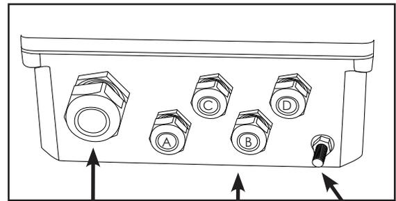
Hybrid Trunk Cable Entry Port      4 - Hybrid Tail Entry Port      Ground
