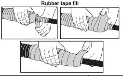
• Prepare the cable by removing any cable markers and drying the cable and Connectors. Starting at 2" (51mm) from the feeder connector, wrap the connection with a layer of 3/4" (19mm) plastic tape. Overlap the tape to half-width and extend the wrapping 2" (51mm) beyond the jumper connector or plastic strain relief of a jumper. NOTE: Do not remove the jumper strain relief.
