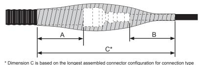
$\mathbf{5}$  Wrap the connection with a layer of the 2" (51mm) tape and then three continuous layers of the 3/4" (19 mm) plastic tape. Overlap each tape to half-width and extend the wrapping 2" (51mm) beyond the previous tape. Do not stretch the tape.
