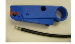
Peel the foam from the cable with fingers or pliers.
