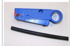
2 Hold the tool, depress the lever. Insert the cable across the cartridge to the edge of the tool, in the direction of the arrow.
