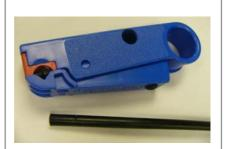
Insert the cable into the slitter blade hole in the side of the tool. Line the slitter blade up with the rotational cut.
