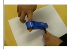
Squeeze the tool open and remove it from the cable.
