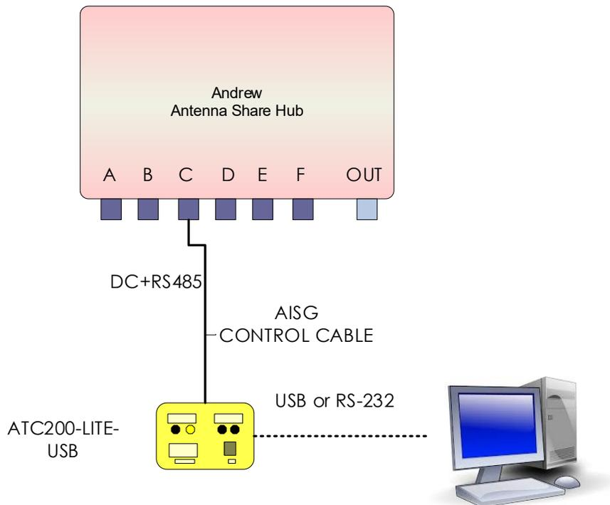
Figure 6 ATC200-LITE-USB connected to ANDREW Antenna Sharing Hub on control port C.
