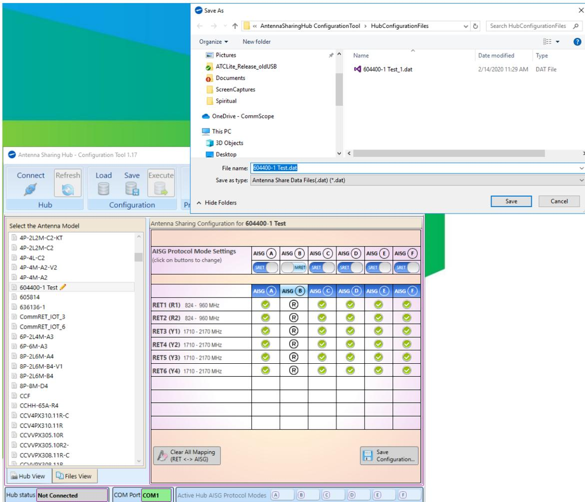
Figure 28 Saving Antenna Sharing Configuration .dat files.
