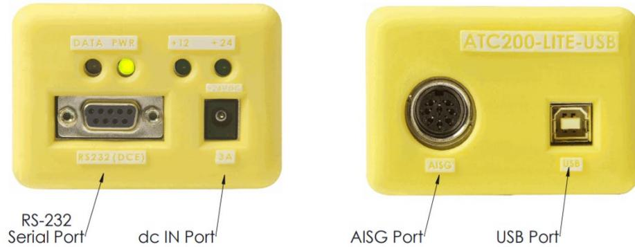
Figure 7 ATC200-LITE-USB Controller End Panels
