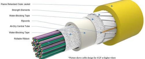
\*Picture shows cable design for 432F or higher where ribbons are bundled in groups of 144F per bundle. \*144F & 288F count designs use water blocking threads rather than a water blocking tape inside the buffer tube.
