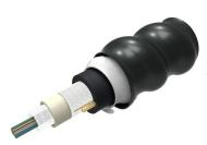
Fiber Indoor/outdoor Cable, Interlocking Armored, Low Smoke Zero Halogen (LSZH), Riser-Rated, 144 fiber, Gel-Free, Central Tube Ribbon, Singlemode G.652.D and G.657.A1, Feet jacket marking, Black jacket color
