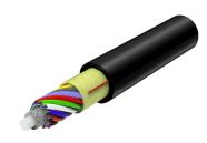
Fiber indoor/outdoor cable, LSZH, 96 fiber Microsheath, Tube Colours as per DIN/VDE 0888, Singlemode G.657.A1, Gel-free, Meters jacket marking, Black jacket color, Dca flame rating
