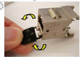
... Check both sides are fully inserted and the dust cover is functional and rotates...
