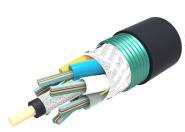
Fiber OSP cable, Steel Armored, Gel-Filled Loose Tube Ribbon, 432 fiber, Singlemode G.657.A2, Feet jacket marking, Black jacket color
