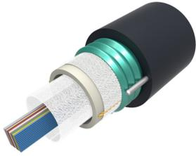
Fiber OSP cable, Steel Armored, Arid-Core, Dry Central Tube Ribbon, 144 fiber, Singlemode G.657.A2, Feet jacket marking, Black jacket color
