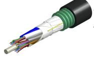
Fiber OSP cable, LightScope ZWP® Mini Single Jacket/Single Armor, 12 fiber, Gel-Filled, Stranded Loose Tube, Singlemode G.657.A2, Meters jacket marking, Black jacket color
