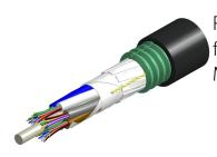
Fiber OSP cable, LightScope ZWP® Mini Single Jacket/Single Armor, 48 fiber, Gel-Filled, Stranded Loose Tube, Singlemode G.652.D and G.657.A1, Meter jacket marking, Black jacket color
