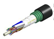
Fiber OSP cable, LightScope ZWP® Mini Single Jacket/Single Armor, 24 fiber, Gel-Filled, Stranded Loose Tube, Singlemode G.652.D and G.657.A1, Meters jacket marking, Black jacket color
