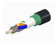
Fiber indoor/outdoor cable, LightSCOPE® Indoor/Outdoor, Single Jacket /Single Armor, Low Smoke Zero Halogen (LSZH), Singlemode G.652.D and G.657.A1, 72 fiber, Gel Filled, Stranded Loose Tube, Feet jacket marking, Black jacket color, Cca flame rating
