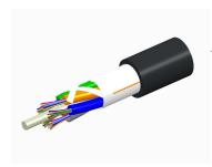
Fiber OSP cable, LightScope ZWP® Single Jacket All-Dielectric, 228 fiber, Gel-Free, Stranded Loose Tube, Singlemode G.652.D and G.657.Al, Feet jacket marking, Black jacket color
