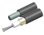
Fiber outdoor drop cable, LightScope ZWP® Self-Supporting Non-Armored Figure-8, Singlemode G.652.D and G.657.A1, 6 fiber Arid Core construction with 0.109 in messenger, Gel-filled, central loose tube, Feet jacket marking, Black jacket color
