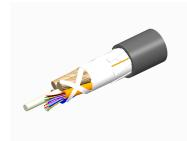
Fiber indoor/outdoor cable, LightScope ZWP®, Single Jacket All-Dielectric, Plenum Rated, Gel-Free, Singlemode G.652.D and G.657.Al, 12 fiber, Stranded Loose Tube, PVDF jacket, Feet jacket marking, Black jacket color
