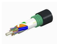
Fiber OSP cable, LightScope ZWP® Single Jacket/Single Armor, 56 fiber, Gel-Free, Stranded Loose Tube, Singlemode G.652.D and G.657.A1, Meters jacket marking, Black jacket color
