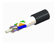
Fiber OSP cable, TeraSPEED® Single Jacket All-Dielectric, Gel-Free, 96 fiber, Stranded Loose Tube, Singlemode G.652.D and G.657.Al, Meters jacket marking, Black jacket color
