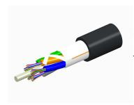
Fiber OSP cable, LightScope ZWP® Single Jacket All-Dielectric, 72 fiber, Gel-Free, Stranded Loose Tube, Singlemode G.652.D and G.657.Al, Meter jacket marking, Black jacket color
