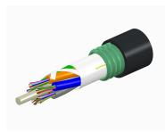
Fiber OSP cable, LightScope ZWP® Single Jacket/Single Armor, Gel-Free, 6 fibers, Stranded Loose Tube, Singlemode G.652.D and G.657.Al, Meters jacket marking, Black jacket color
