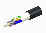
Fiber OSP cable, LightScope ZWP® Single Jacket All-Dielectric, 12 fiber, Gel-Free, Stranded Loose Tube, Singlemode G.652.D and G.657.A1, Meter jacket marking, Black jacket color
