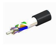
Fiber OSP cable, LightScope ZWP® Single Jacket All-Dielectric, 120 fiber, Gel-Free, Stranded Loose Tube, Singlemode G.652.D and G.657.A1, Feet jacket marking, Black jacket color
