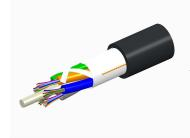
Fiber OSP cable, LightScope ZWP® Single Jacket All-Dielectric, 72 fiber, Gel-Free, Stranded Loose Tube, Singlemode G.652.D and G.657.A1, Feet jacket marking, Black jacket color
