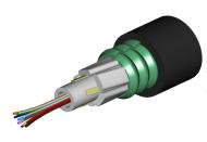
Fiber drop cable, LightScope ZWP® Single Jacket Single Armor Outdoor Drop Cable, 4 fiber Arid Core construction, central loose tube, Gel-filled, Singlemode G.652.D and G.657.Al, Meter jacket marking, Black jacket color
