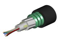
Fiber drop cable, LightScope ZWP® Single Jacket Single Armor Outdoor Drop Cable, 12 fiber Arid Core construction, central loose tube, Gel-filled, Singlemode G.652.D and G.657.A1, Custom jacket marking, Black jacket color
