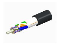
Fiber OSP cable, LightScope ZWP® Single Jacket All-Dielectric, 108 fiber, Gel-Free, Stranded Loose Tube, Singlemode G.652.D and G.657.Al, Meters jacket marking, Black jacket color
